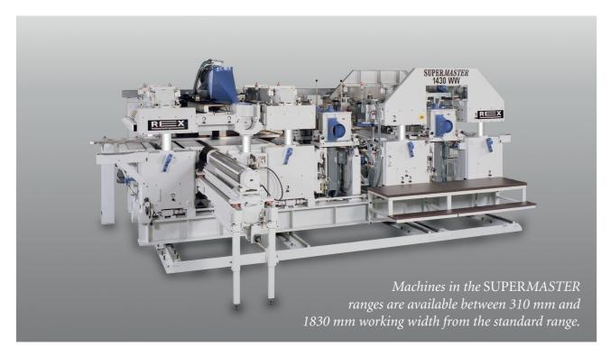
REX SUPERMASTER 1430-WW with 10 working spindles, left-hand version, REX exchangeable cutter blocks, 1430 mm working width, directly-driven vertical spindles, machine can be completely moved to use total working width even with small workpieces.
