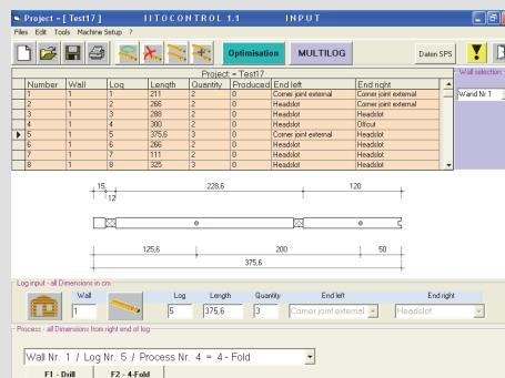
The list of the workpieces at the IITO Software is automatically optimized to a Multilog list with multiple lengths (Optimized Exploitation of the Wood length) for the production.
