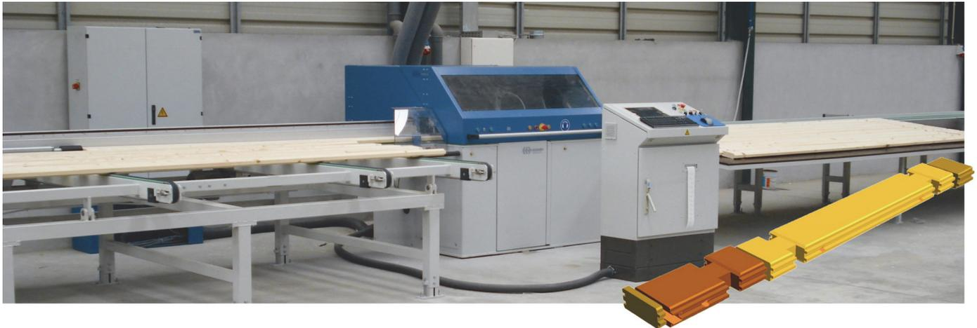
Fully automated Loghouse milling machine Blockhausfräse BL100A for economic production of components used in modern log cabin construction.
