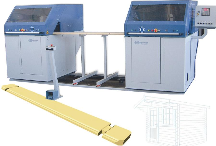
The hydro pneumatic feeding system with an express traverse, allows the creation of a four-fold corner joint only in a few seconds! High performance spindle drives and climb milling ensures a clean cut milling contour without being frayed.
