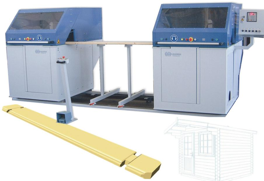
Double end Log cabin milling machine Blockhausfräse BL Twin for serial production of components for garden log Cabins.
