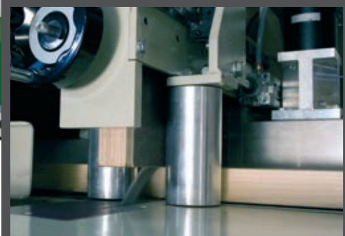
► Heavy-duty top pressure unit and intelligent side rollers gives an exact cut and positioning of the workpieces during cross-cutting.
