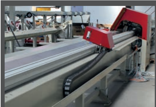
► The push arm is controlled by a servo driven linear module for high capacity and cut accuracy with a minimum of maintenance.
