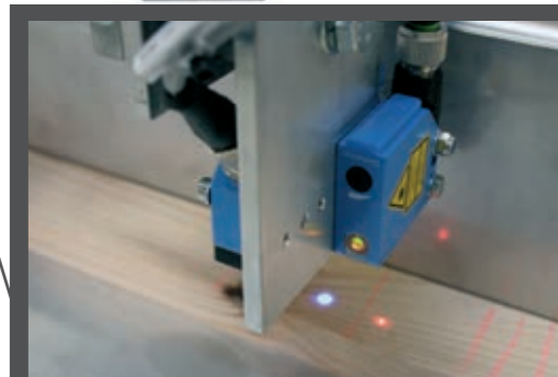
► With a return speed of 310 m/min (1,017 ft/min) the sensors registers defects, quality and measures the board length.
