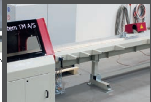
► High-speed push arm with a feeding speed of 140 m/min (460 ft/min) and return speed of 310 m/min (1,017 ft/min).
