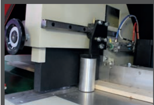
► High-precision cut accuracy. Push positioning accuracy of +/- 0.1 mm (0.004").
